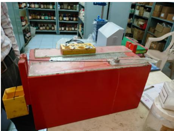
Figure 4. Spreadability test setup for evaluation of clove oil-loaded niosomal gel using the glass slide method.
