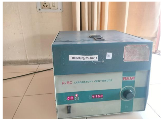
Figure 6. REMI R-8C laboratory centrifuge used for the separation of free and encapsulated clove oil.
