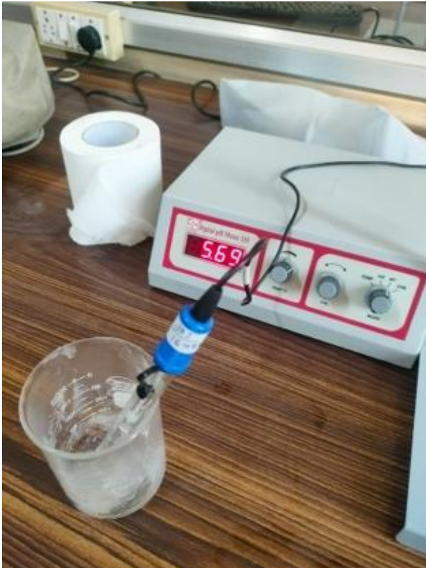
Figure 3. Measurement of pH of clove oil-loaded niosomal gel using a digital pH meter.
